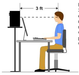
Earthquake Sound suggests placing the SM6BT monitors at least 3 feet away to reduce distortion by reflection and di raction. Because high frequencies are primarily directional, to achieve the most precise monitoring, the SM6BTs should be placed so that the ribbon tweeters are approximately the same height as your ears when seated at your listening position. To attain the optimized performance, you may angle the monitors to aim towards your ears when in your listening position.
