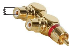
RCA with 600Ω 1/4W resistor between the positive & ground
