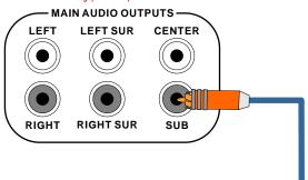
Usually one RCA has enough signal to drive the IQ amplifier to its full output. However, in some cases where signal is too low for the IQ amp to produce its full output, you may use a "Y" connector to increase the amp's sensitivity.
