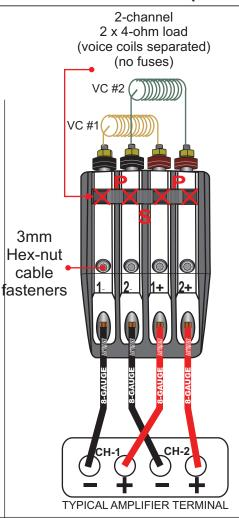
This diagram shows the PSP terminal in a 4-ohm configuration (the two voice coils are separated). No fuses are used in this configuration, the voice coils are powered up separately.
