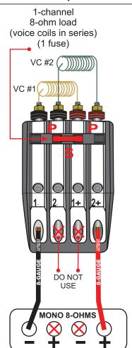
The diagram - on the right side-displays the PSP in an 8-ohm mode. You will notice that there is only one fuse in the center of the fuse placement area. The voice coils are wired in series. Insert the negative speaker wire to the far left insert and one positive to the far right insert.
